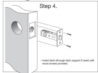
Carefully follow these instructions when installing. Screws to be tightened to a recommended 2.5Nm torque.
